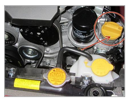
Refill the engine with oil. Do not over-fill. Add the amount that is suggested in the owners manual.
