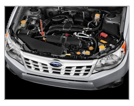
Start the engine. Verify there are no leaks. Then drive your Subaru to a flat place. Shut off engine. Open the hood and take out the engine oil dipstick. Wipe with a paper towel. Reinsert all the way. Then take out again. Make sure the oil is full. Add more if necessary!
