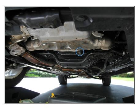
Before refiling the engine with 0W-20 oil, reinstall and tighten the drain plug. Don't over tighten!
