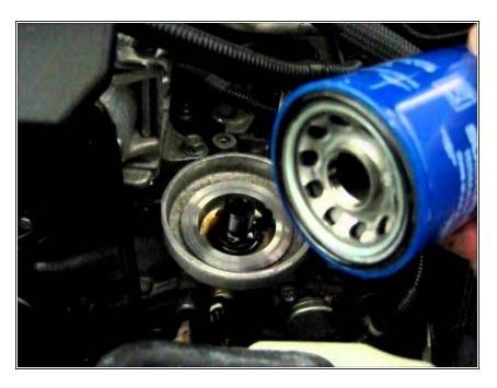
• As the oil drains, get out from under your car and take off oil filter. Make sure the old gasket comes off with old oil filter. If not, remove from engine. Then add some oil to the gasket of the new filter via your finger. Then scew onto engine but do not over tighten.
