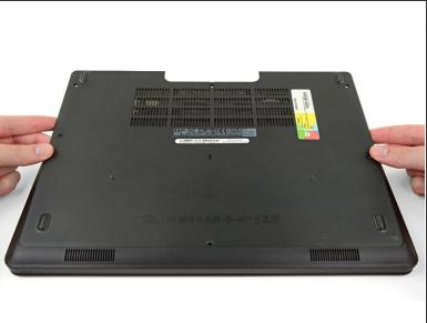
When reinstalling the lower case, make sure you slide the bottom edge (the edge without the cutout) into place first before snapping the rest of the clips shut.
