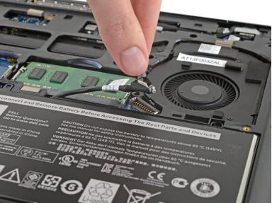
Pull up on the battery connector's pull tab to disconnect the battery.
