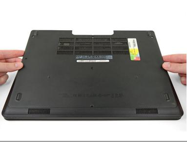
When reinstalling the lower case, make sure you slide the bottom edge (the edge without the cutout) into place first before snapping the rest of the clips shut.
