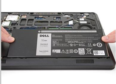
When installing your new battery, slide the bottom edge in first, and make sure it lays flat before you proceed to reinsert the screws or reconnect it.
