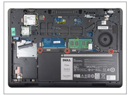
Remove the three 5.6 mm Philips #0 screws from the top edge of the battery.
