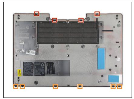
This photo shows the location of the ten clips that hold the lower case in place. Take note of the location of
