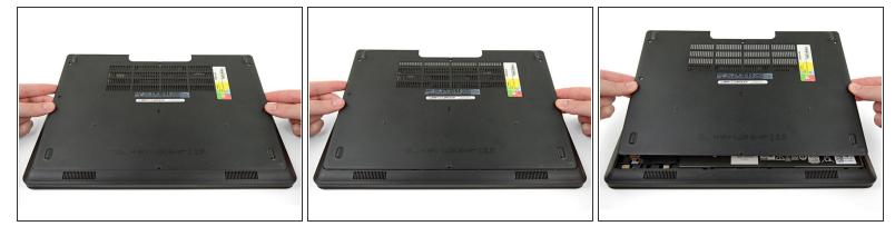
Slide the lower case upward and remove it.
