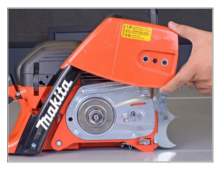
Remove the sprocket guard plate.
