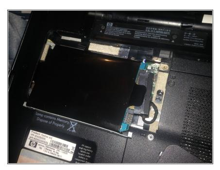
Remove the SATA cable from the hard drive, then remove the hard drive.
