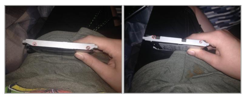
Remove the screws from the hard drive enclosure.
