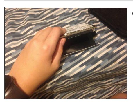
Remove the Hard Drive from the enclosure
