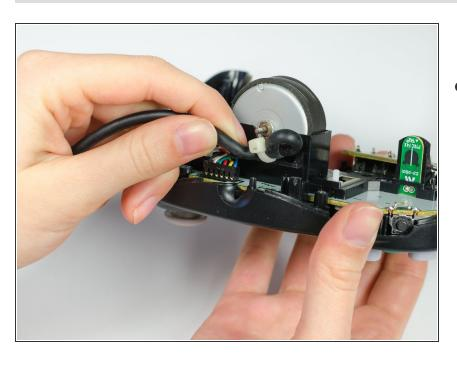
Carefully unhook the cable that is looped around the peg.
