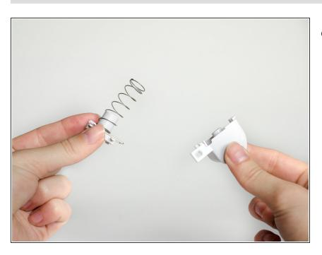
Pull the metal clip from the trigger.
