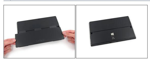
• Gently pull the kickstand away from the device. This will release the three tabs from the slots on the back of the device.
