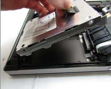
Remove the silver metal cover by pulling straight up on the black tab.
