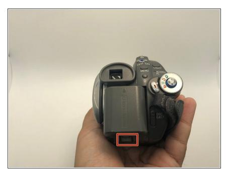
Slide the battery release lever found on the bottom of the camera in the direction of the front of the camera.
