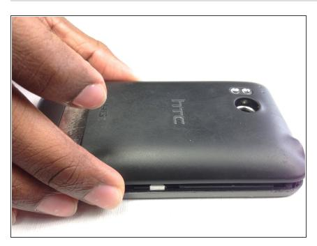
Lift and remove the rear panel.
