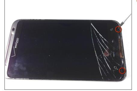
• Remove the two Phillips screws where the plastic cover was.
