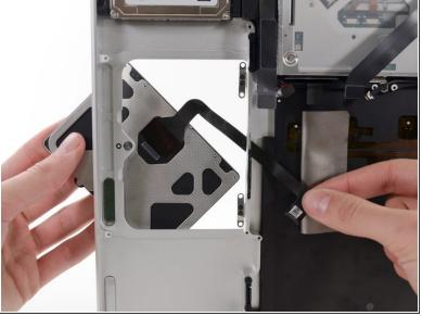
Once the trackpad is free of the upper case, guide the ribbon cable through the slot cut in the upper case.
