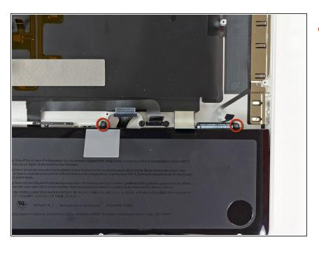
Remove the two 7.5 mm (7.2 mm) Tri-point screws securing the battery to the upper case.
