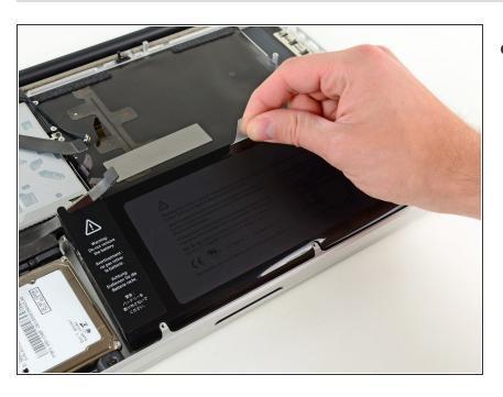
Use the attached plastic pull tab to remove the battery from the upper case.
