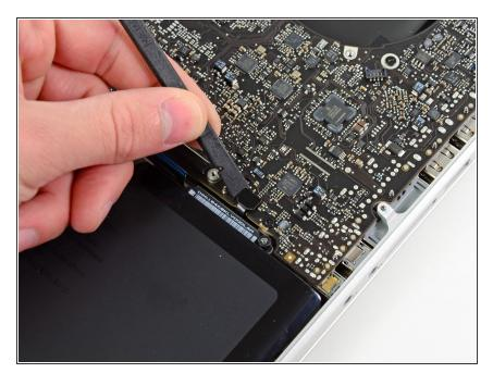
Use the flat end of a spudger to lift the battery indicator connector up and out of its socket on the logic board.
