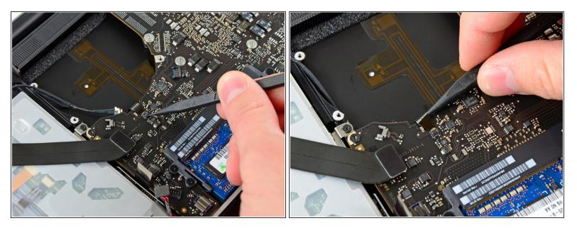
Use the tip of a spudger to flip up the retaining flap on the keyboard backlight ribbon cable ZIF socket.
