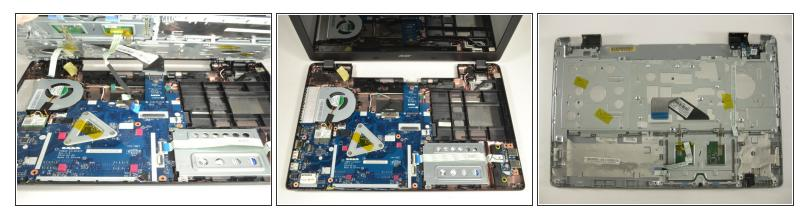
Once all three ribbon cables are disconnected, lift off the top cover with the keyboard and touchpad.
