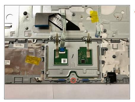
Remove the screw at the bottom of the track pad using the Phillips #0 screwdriver.
