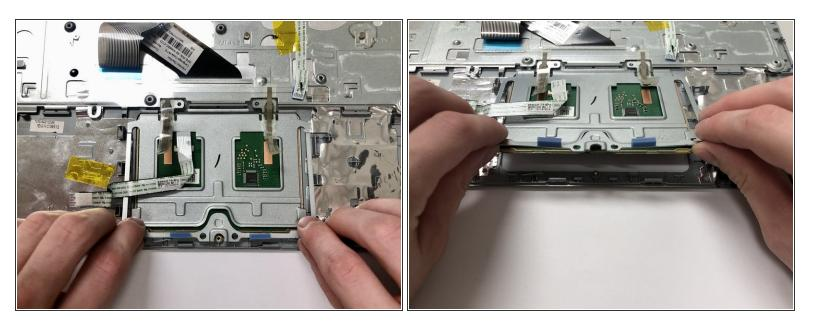
• Pop the track pad out of of the keyboard casing and remove it from the device.
