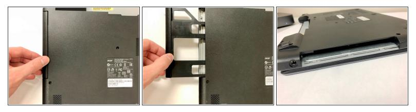
• Slide out the old optical drive and remove it from the device.
