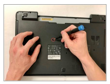
Remove the single screw that holds the optical drive in place using the Phillips #0 screwdriver.
