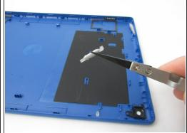
Use tweezers to remove and pick up the button carefully.
