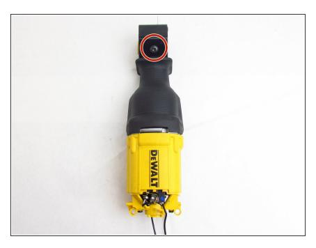
Remove the large screw from the locking area of the device using a Phillips #2 screwdriver.
