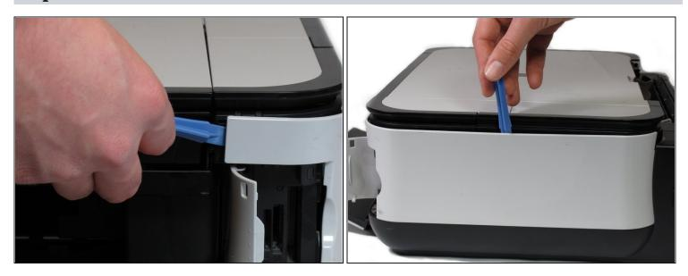
Pry open the side cover with the plastic opening tool.
