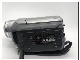
Remove one 5mm screw on the bottom side of the camera with a Phillips #0 screwdriver.
