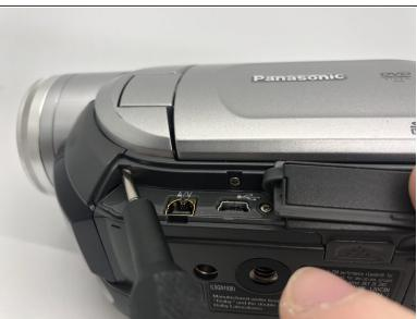
• Remove one 5mm screw inside the side port with your Phillips #0 screwdriver.
