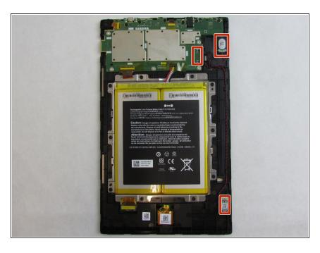
After removing the top case identify the speakers and wires connected to the motherboard.
