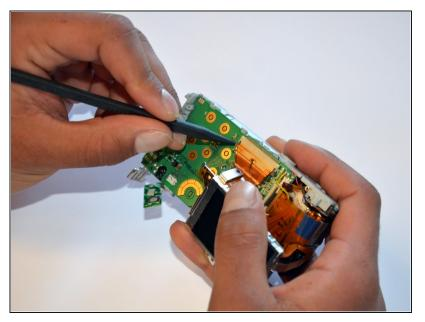
Using a spudger, lift the grey tabs to allow the ribbon to slide out.
