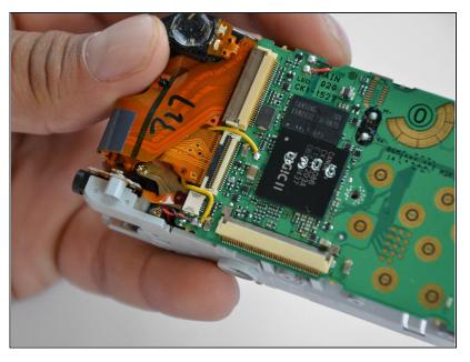
All that is required is to unsolder the few remaining wires. Then, the motherboard will be ready to be replaced!
