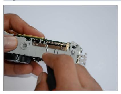
Remove the 5mm Phillips #00 screw that holds the metal piece to the bottom of the camera.
