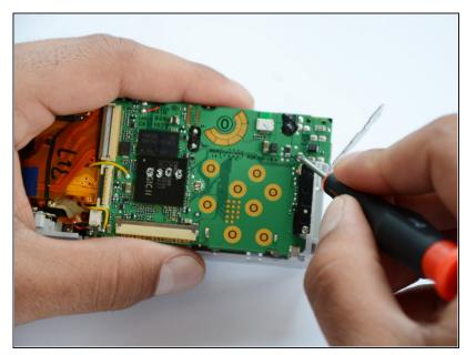
Remove the 5mm Phillips #00 screw located above the small black piece on the right side of the mother board.
