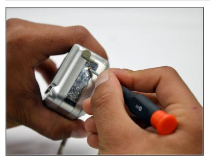
Remove the 4mm Phillips #00 screw that is located on the left side of the camera, if the display screen is facing you.
