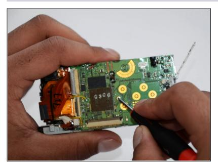
Remove the 5mm Phillips #00 screw in the middle of the motherboard.
