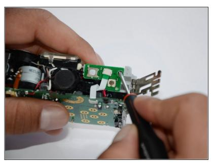
Remove the 5mm Phillips #00 screw that is located on the top of camera.
