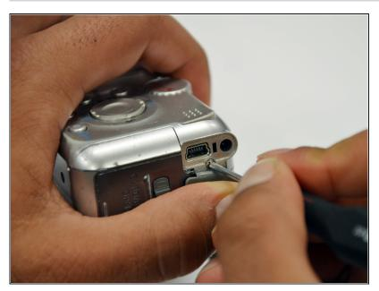
• Take out the 4mm Phillips #00 screw under the rubber flap on the right end of the camera.
