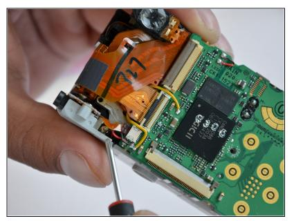
Remove the 5mm Phillips #00 screw near the bottom left of the motherboard.
