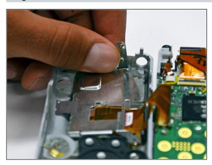
• Gently lift the LCD screen off of the front casing by pulling up a tab on the side of the camera.
