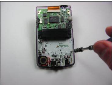
Using the Phillips #1 screwdriver, remove the 3 screws shown in the picture.
