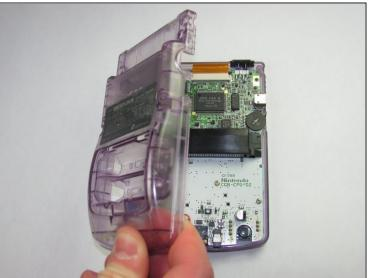
• Gently lift and separate the back housing from the rest of the device. Now you've got the back housing out!
