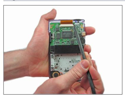
• Push up on the tabs on either side of the ribbon with a spudger.
