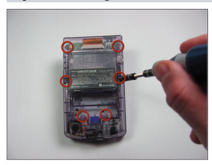
Using a Y1 screwdriver, remove the six screws on the back of the device as pictured. The bottom two screws are located inside of the battery compartment.
