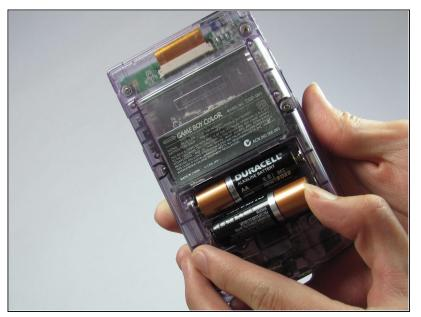
• Remove the batteries from the battery compartment.
