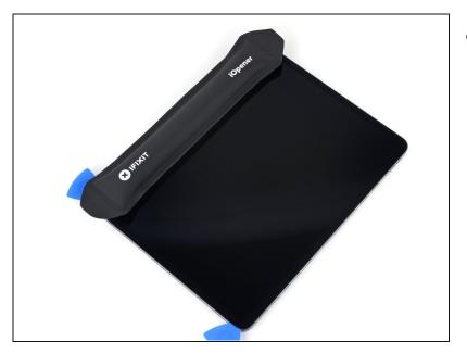
Apply a heated iOpener to the left edge of the screen for two minutes.
