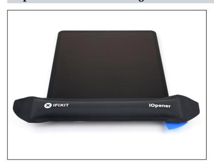
Apply a heated iOpener to the bottom edge of the screen for two minutes.
