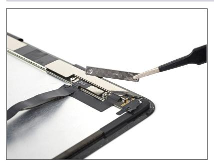
Remove the display cable bracket.
