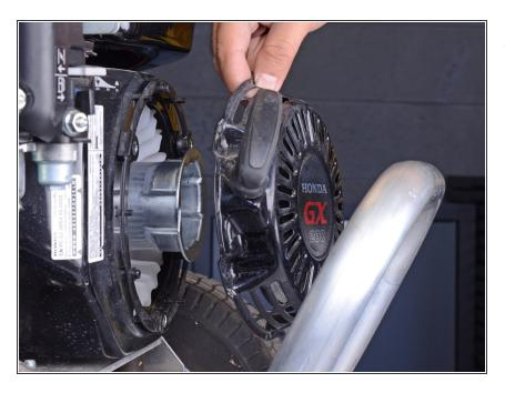
Remove the recoil starter assembly.
