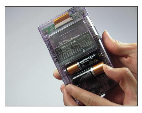
Remove the batteries from the battery compartment.
