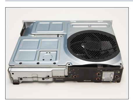
Flip the metal enclosure so that the fan cover is on top.
