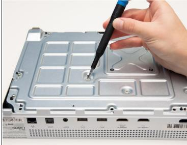
Remove the two 10mm screws, labeled C3 and C4, attaching the plastic hard drive case to the metal chassis with the Torx T10 Security screwdriver.
