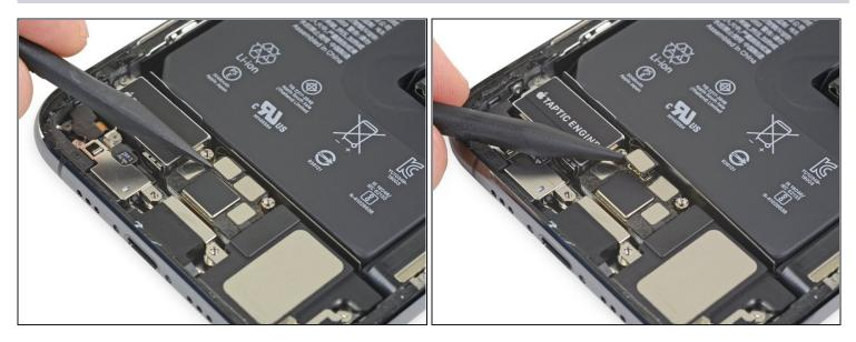
• Use a spudger to disconnect the lower battery flex cable by prying it straight up from its socket.
