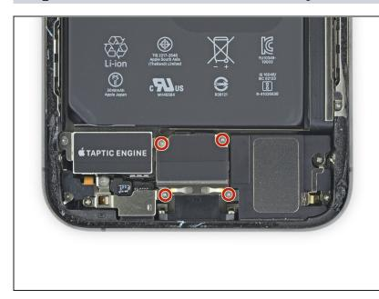
• Use a Y000 driver to remove the four 1.5 mm screws securing the lower battery connector cover.
