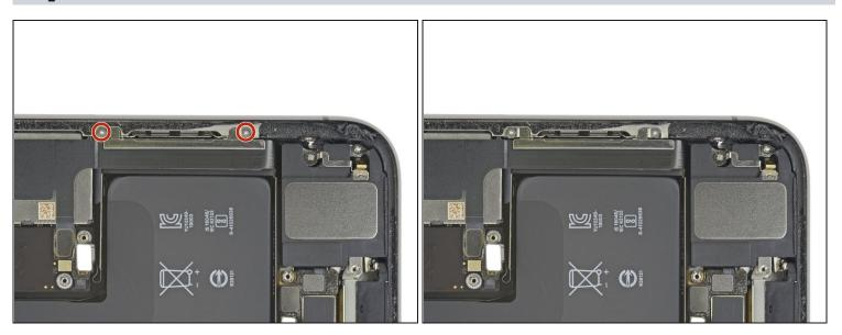
• Use a Y000 driver to remove the two 1.4 mm screws securing the Lightning flex cable bracket.
