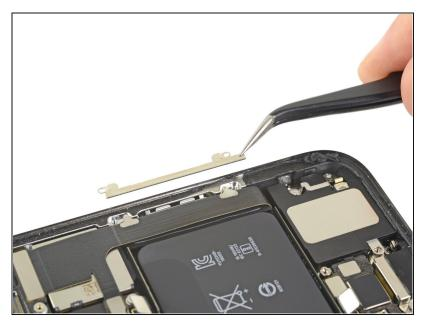
• Remove the flex cable bracket.
