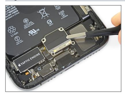
• Remove the lower battery connector cover.
