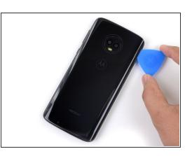
Slide the pick along the right edge of the rear glass to separate the adhesive underneath.
