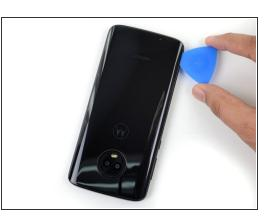
Slide a pick along the left edge of the phone to slice through the rear glass adhesive.
