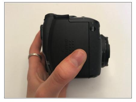
Locate the battery compartment cover on the right hand side of the camera. The cover features the text: "CF/BATT.OPEN".
