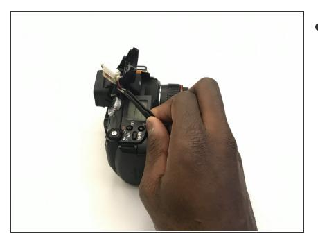
• Cut the flash and capacitor cables with a wire cutter.
