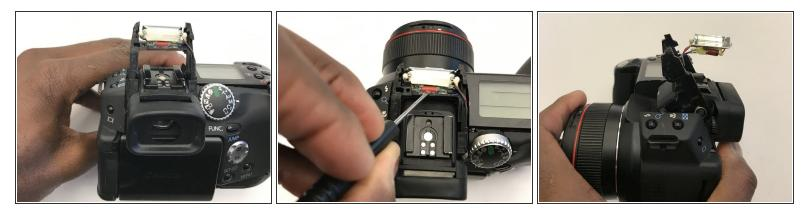
• Use the nylon spudger to dislodge the flash bulb and capacitor from the housing.
