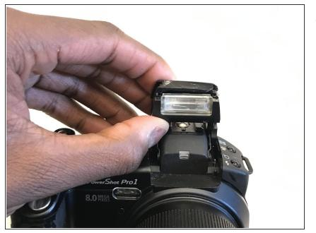
Use the plastic spudger to remove the upper portion of the flash housing.
