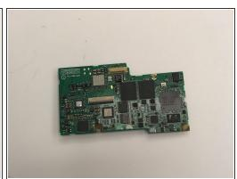
Once detached from all connectors and ribbon cables, remove the motherboard.
