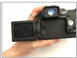
Open the screen to access the underside of the camera.
