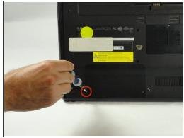
• Use a Phillips #00 screwdriver to remove the two 7.8 mm cover screws on the bottom corners of the panel.
