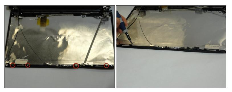
Use a Phillips #00 screwdriver to remove the four 3.15-mm screws at top of the display.
