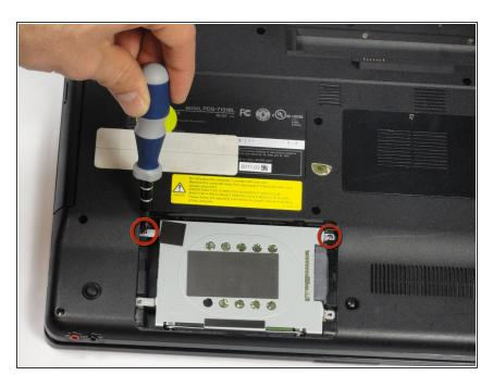
Remove the two remaining 7.8 mm screws using the Phillips #00 screwdriver.
