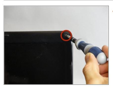
Use a Phillips #00 screwdriver to remove the four 5.75-mm screws under the plastic covers.
