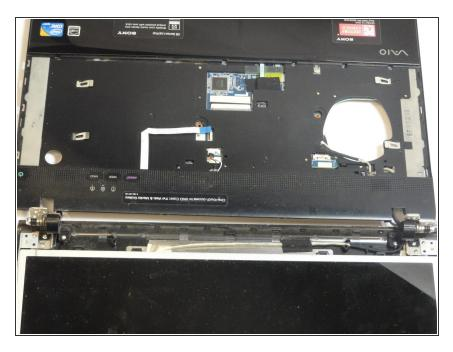
Gently pull out the base and place it with the keyboard side up under the display.
