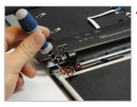
Use a Phillips #00 screwdriver to remove the four 5.65-mm screws on each bottom corner of the display.
