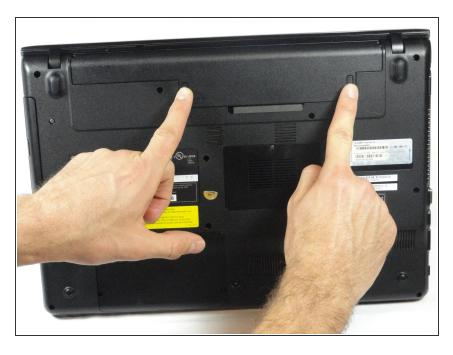
To release the battery, hold both the release button and the unlock button at the same time.
