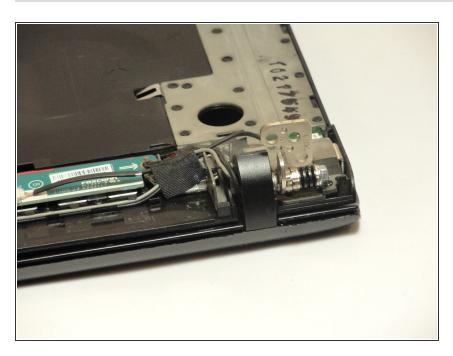
Lift the metal hinges on each corner to a 90° angle.
