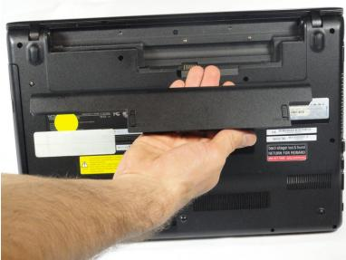
Remove the battery out from the notch while continuing to hold the release button.
