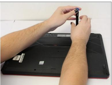
Remove the eleven Phillips #0 screws that secure the back cover.
