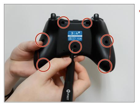
Remove the seven 12mm JIS #00 screws that hold the back panel in place.
