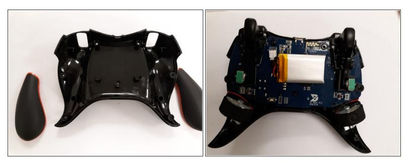
• Lift up on the back panel of the ZD-N Plus to remove it from the rest of the controller.
