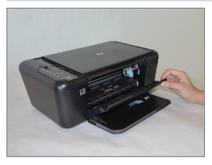
• Open the front access panel by placing your finger in the front slot and pulling gently.
