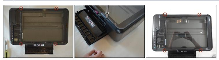
• Remove the **four** 9mm T10 Torx screws on the top.
