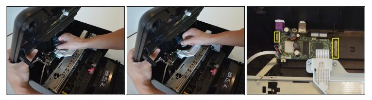
• Remove the **two** cables by gripping each one close to their connection ports on the motherboard and gently disconnecting them.
