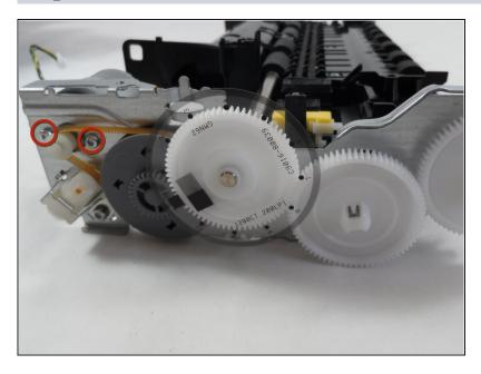
• Remove the **two** 6mm torx screws using a T9 Torx bit.
