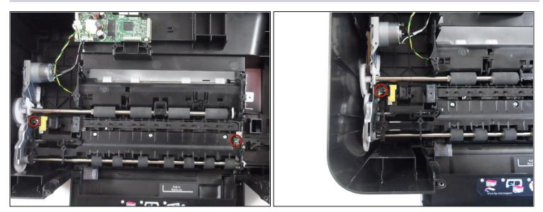
• Remove the **two** 9mm Torx screws in order to detach the roller assembly from the system.
