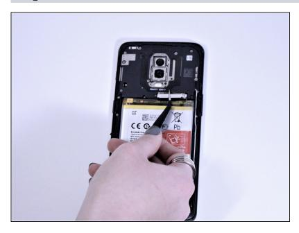
Using tweezers, carefully remove the small metal bracket covering the battery connector.
