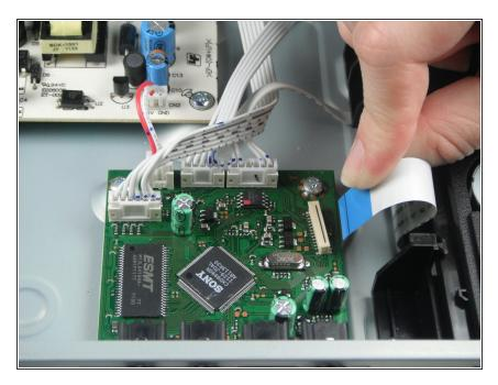
Remove the blue tape from the processing board by gently pulling upward.
