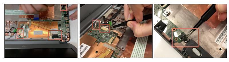
Carefully remove the 4 connections.
