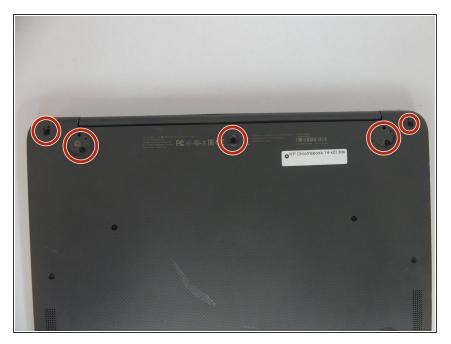
Remove the five 6mm screws located under the removed pads using Phillips #00 screwdriver.
