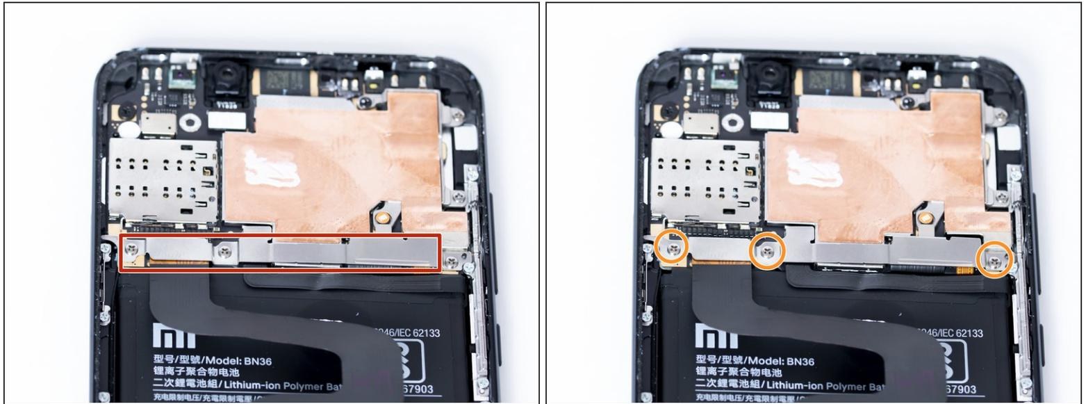
**⚠** When removing the ribbon cable and installing the new one take special care to not bend or fold the cable too much as this can cause damage to the cable itself.
