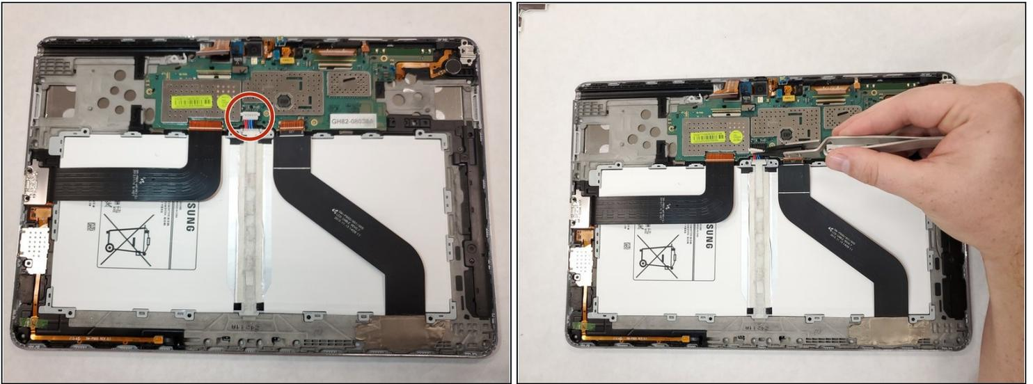
⚠ Potential damage to the motherboard could occur without supporting the black motherboard connector as the white cable connector is being removed.
