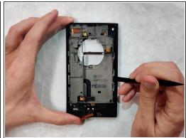
Insert the spudger on the edges of the base and lift up.
