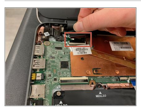
Pull the ribbon cable out of socket.
