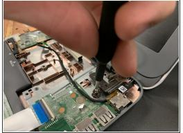
Use a Phillips #00 screwdriver to remove the two 6mm screws located at the upper left and right corners.
