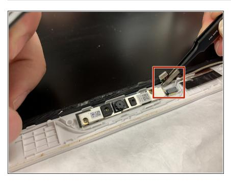
Using tweezers, gently remove the connection hold the camera in place.
