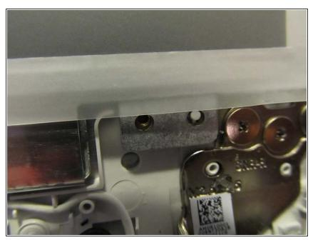
Lift the screen back into place. Use the plastic rivets to get the screen into the proper place prior to screwing the screws back in.
