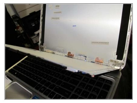
• With the 4 screws removed, you can now slowly pull the screen off, rotating it towards the keyboard. You can lay it flat on the keys, since the next step is to unplug the LCD cable.
