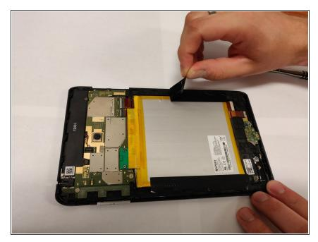
Once you remove the backing of the Verizon Ellipsis 8, gently use the spudger to lift one side of the tape.
