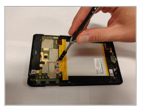
Using a Phillips #00 screwdriver, remove the two 0.1 mm screws on the green bracket.
