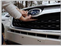
Open the hood of your car by locating and pulling the hood release found on the driver side dash just below (and to the left) of the steering wheel. Then move to the front grill of your car and pull the latch located under the Subaru symbol.
