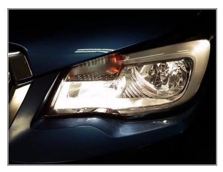
• Make sure you have the correct replacement part. For the specified model, the H11 Headlight Bulb is the stock-standard replacement bulb (found at any automotive store).
