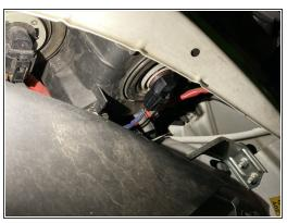
Move to the side that harbors the burnt-out headlight. Locate the headlight assembly which is positioned right behind the headlight itself.
