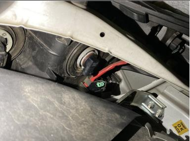
Reach inside the headlight assembly to find the base of the bulb. Push in the release tab ( which is the indention found on the base below the blue tag), then move the power plug downward from the old bulb with above-moderate force.
