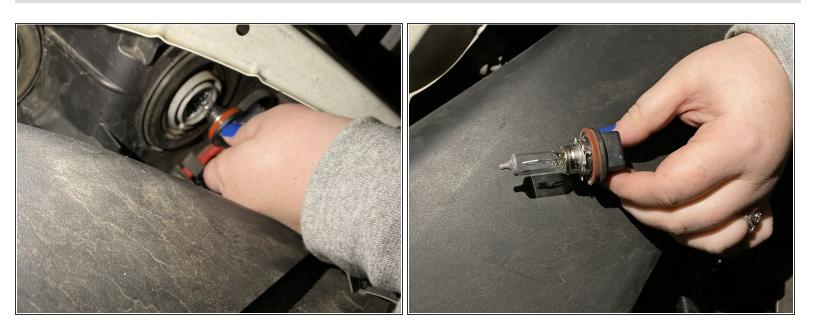
Grab the base of the old bulb and rotate it a quarter length counterclockwise and then you will be able to pull it straight out.
