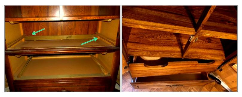
As you can see, the guide tracks that set the drawer in place are no longer attached to the dresser in the correct position.
