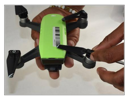
Push down on the propeller that is being replaced.
