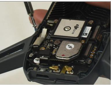
Remove the four 6.0 mm Phillips #000 screws holding the GPS module to the motherboard.
