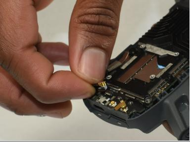
Disconnect two gold antenna next to the internal GPS while removing the motherboard.
