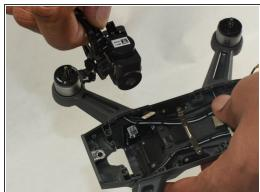
Gently remove the gimbal along with the camera from the top of the device.
