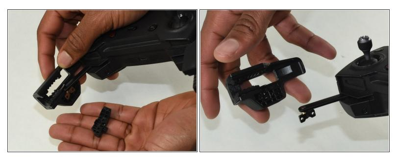
Once both screws are removed, the grip parts come off easily.
