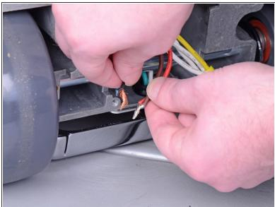
Separate the black copper wire from the brown and red wires.
