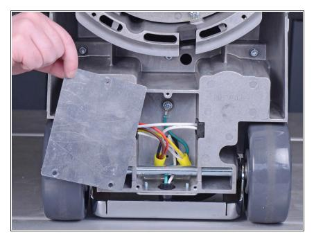
Remove the bottom cover to reveal the wires on the inside.
