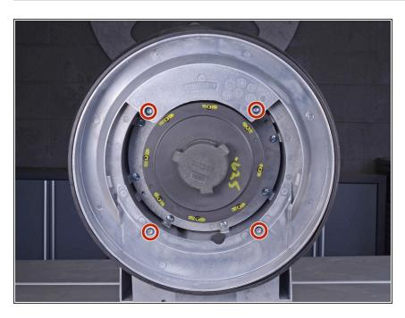
Use a 3/16" hex key or driver bit to remove the four 18.6 mm-long screws securing the shield brush to the bottom of the floor buffer.
