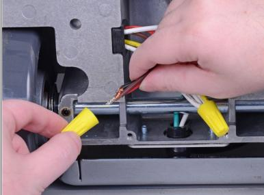
Untwist and remove the yellow wire nuts from the black, brown, and red wires.
