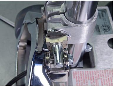
**Re-assembly tip:** The cam lock bolt includes a special square washer. During re-assembly, make sure it's lined up and sits inside the groove of the adjusting arm.
