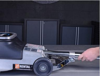
• Loosen the cam lock and tilt the handle all the way back until it rests on your work surface.
