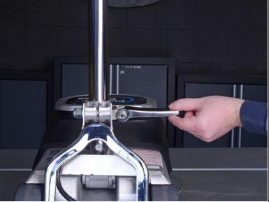
Make sure the handle tube is secured in place by checking that the cam lock is in the locked position.
