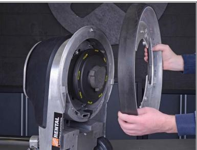
Pull the shield brush straight off the bottom of the floor buffer.
