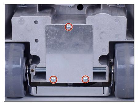
Remove the three 12.6 mm-long Phillips #2 screws securing the bottom cover to the floor buffer.
