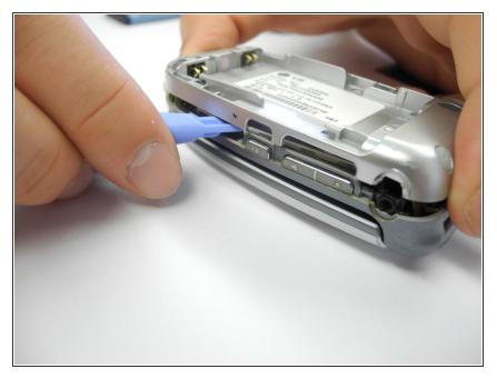
• Using the plastic opening tool, carefully lift the back cover off.
