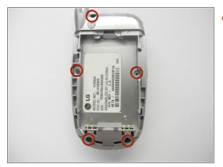
Using a Phillips #0 screwdriver, remove the five screws from the back cover and carefully set them aside.
