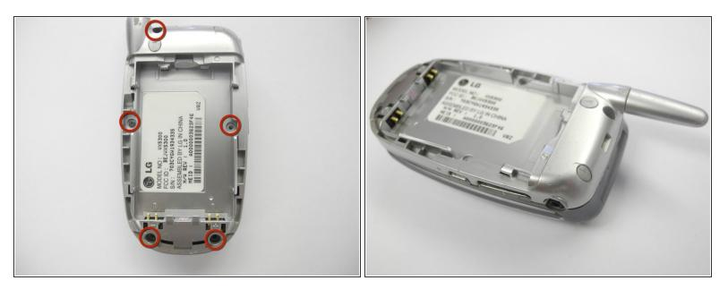
• Place the back cover back on and secure it with the screws.
